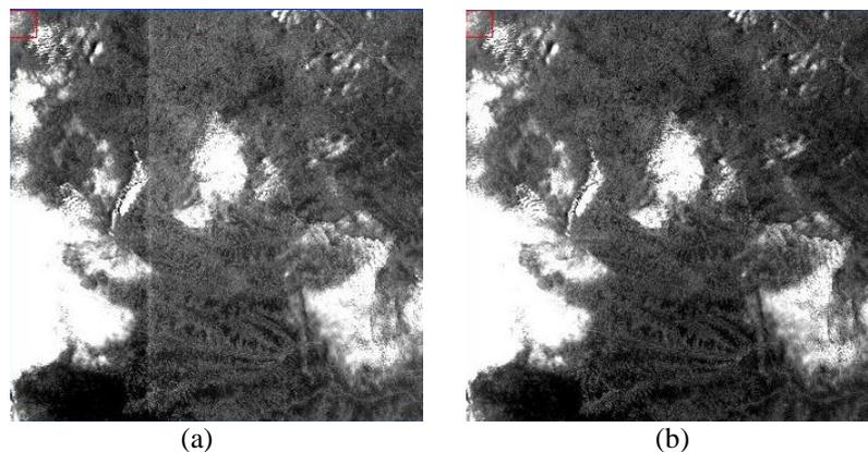
Figure 2: Image of China (a) before and (b) after the relative calibration
